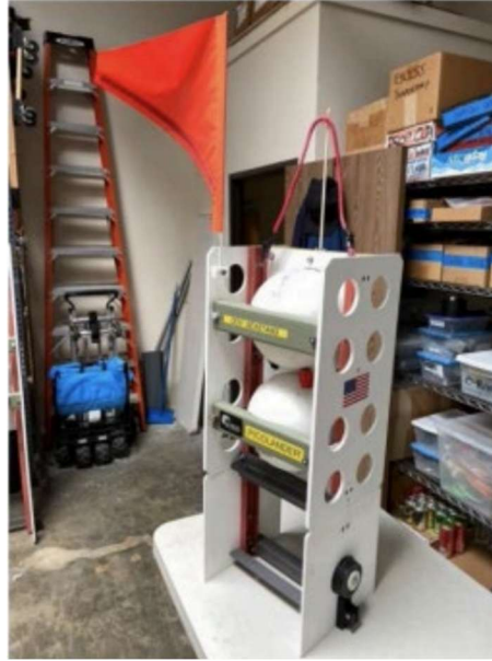
Figure 2: Early BRUV lander built by the Barrel Eye Explorers (Arm, Gariepy, Roberts, & Walsh, 2022)
